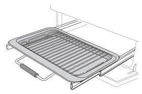
Lift the grill pan clear of the support frame. The support frame is held to the side rails by two clips on each side.
